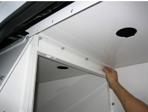
Loosely bolt Passenger-side rear ceilings, Bench/Wall assembly to Middle Bulkhead using 1/4" x 3/4" Carriage bolts and serrated nuts
